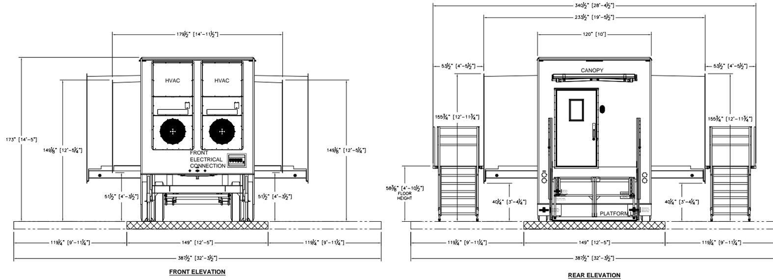
**Figure 5: Front and Rear Side Elevation**
