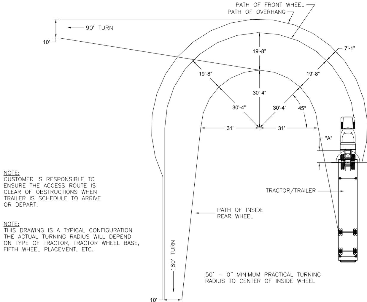
**Figure 6: Turning Requirements**
