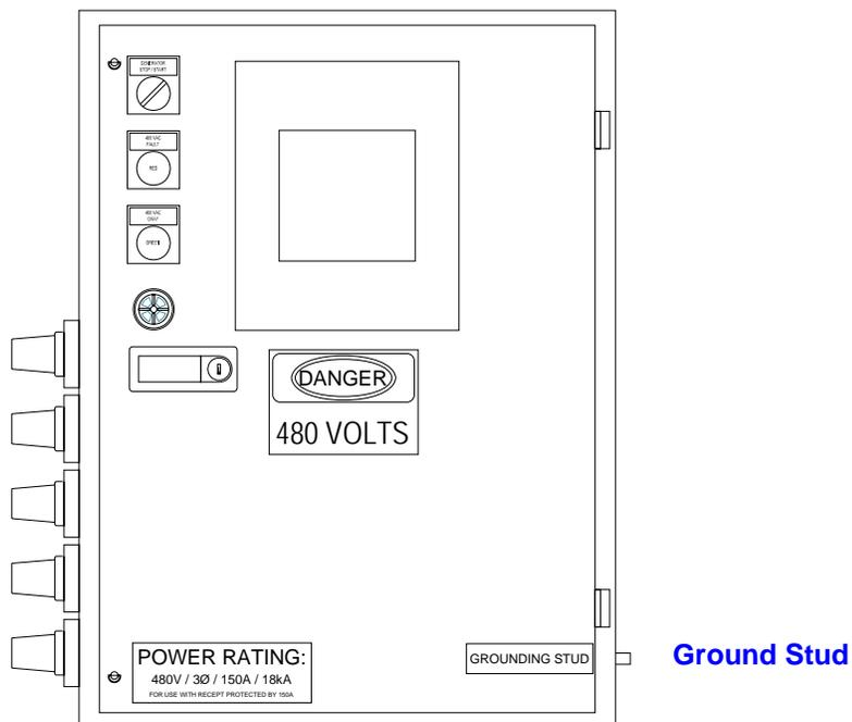
**Figure 1: Automatic Transfer Switch**
