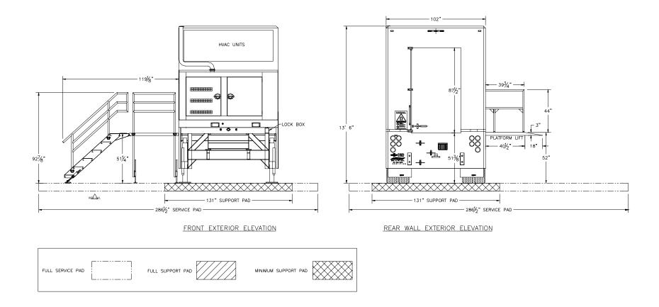
Figure 5: Stair/Lift/Wall Elevation
