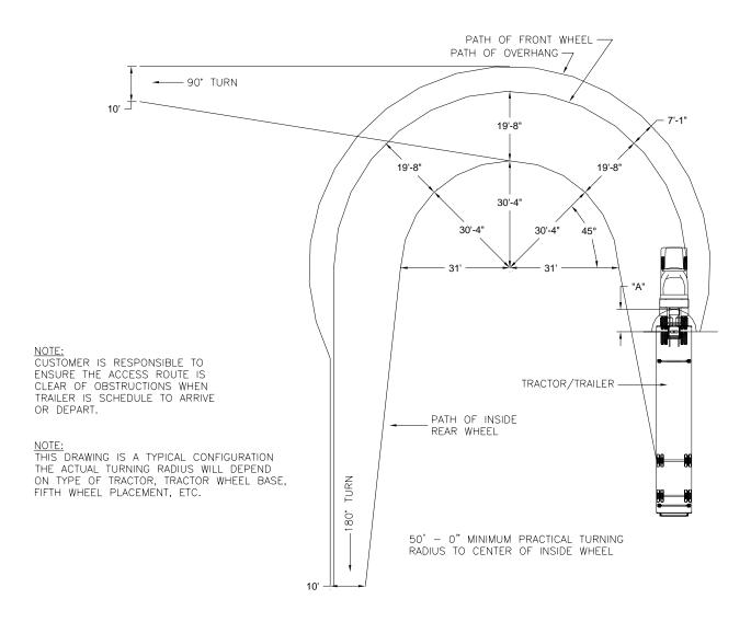
**Figure 6: Turning Requirements**
