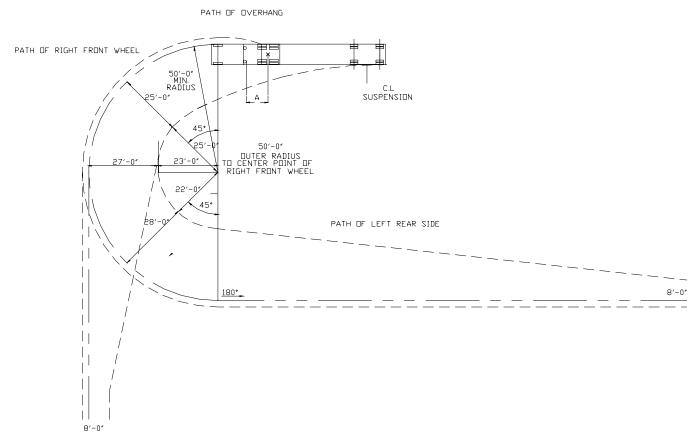
**Figure 7: Turning Requirements**
