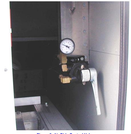
Figure 2: Air Ride Control Valves
