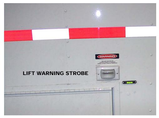
**Figure 63: Lift Transport Warning Strobe**
