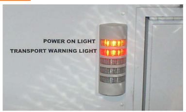
AC Power ON Light and Platform lift Transport Warning Light
