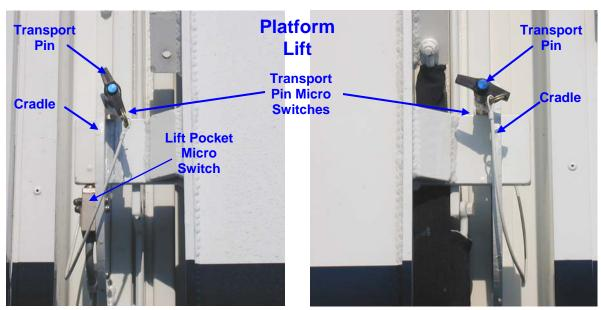
Figure 49: Platform Lift Retaining Cradles
