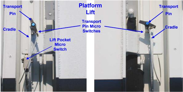
Figure 47: Platform Lift Retaining Cradles
