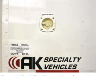
Figure 43: Humidifier External Water Connection
