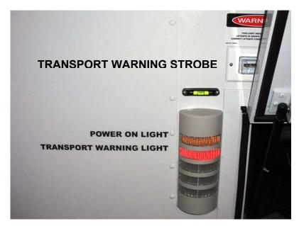
Figure 60: Lift Transport Warning Strobe
