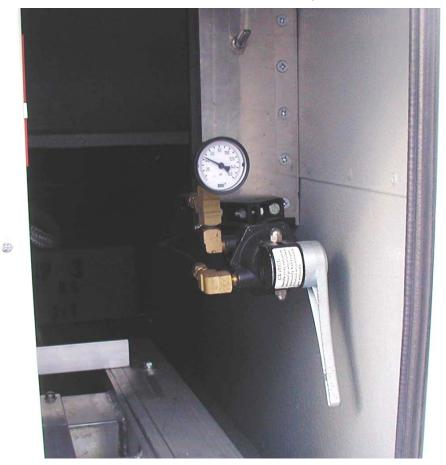
Figure 2: Air Ride Control Valves
