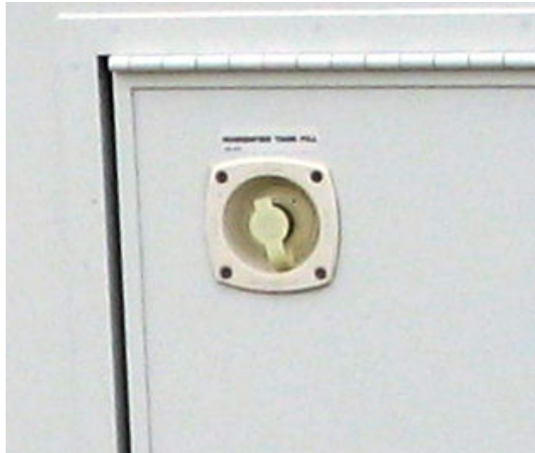
Figure 27: Humidifier Tank Fill
